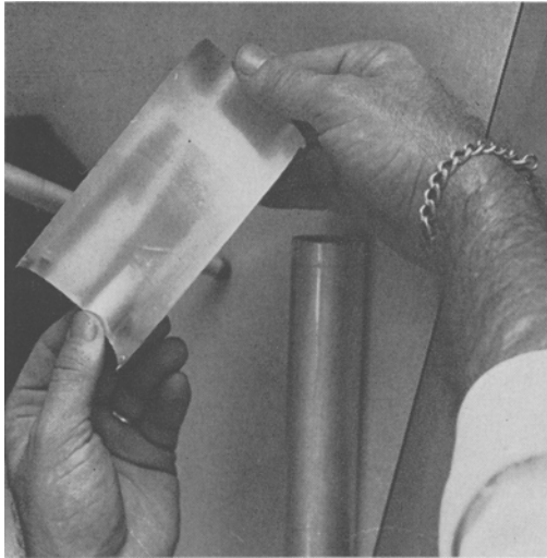
FIG. 4. Dust on the foil liner from the electrostatic air sampler. Dust collects as a stripe near the end of the foil. The dust shown here represents that collected from more than 75 simulated pours.
