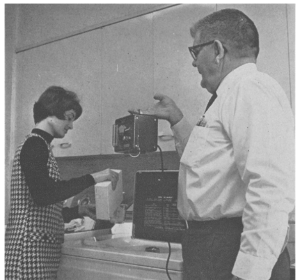
FIG. 6. Collection of dust in consumers' homes. An electrostatic air sampler is held at nose level as housewives pour enzyme laundry product.
